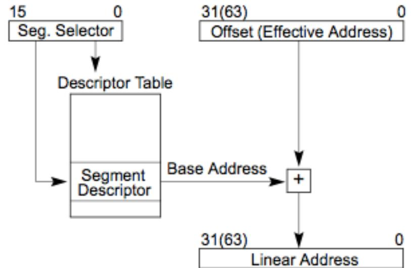
Figure 3-5. Logical Address to Linear Address Translation
