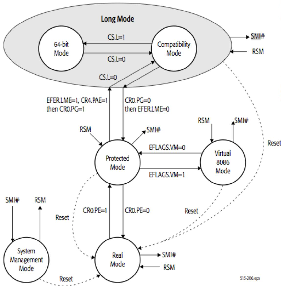
Figure 1-6. Operating Modes of the AMD64 Architecture
