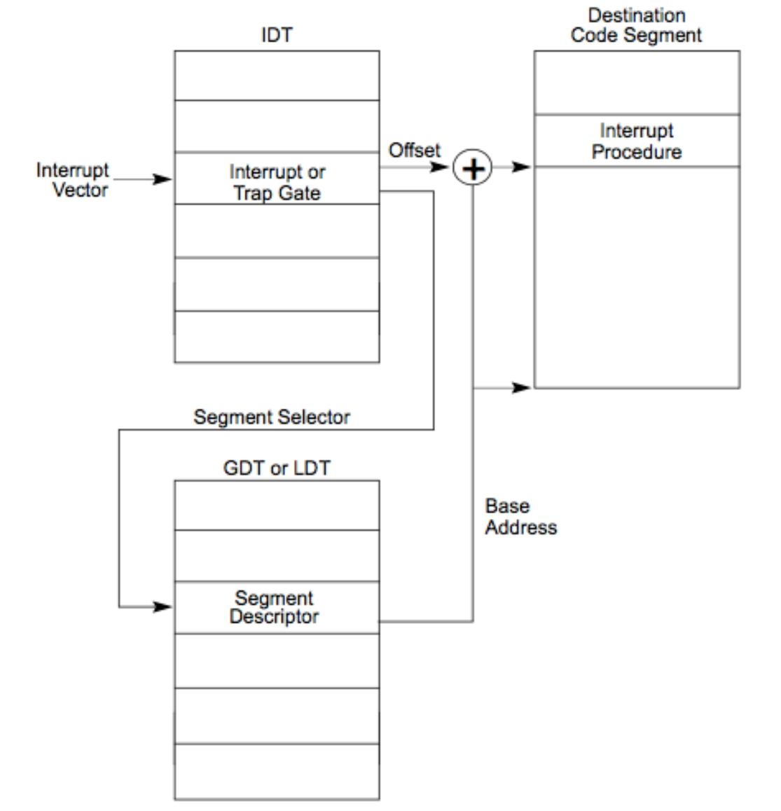
Figure 5-3. Interrupt Procedure Call
