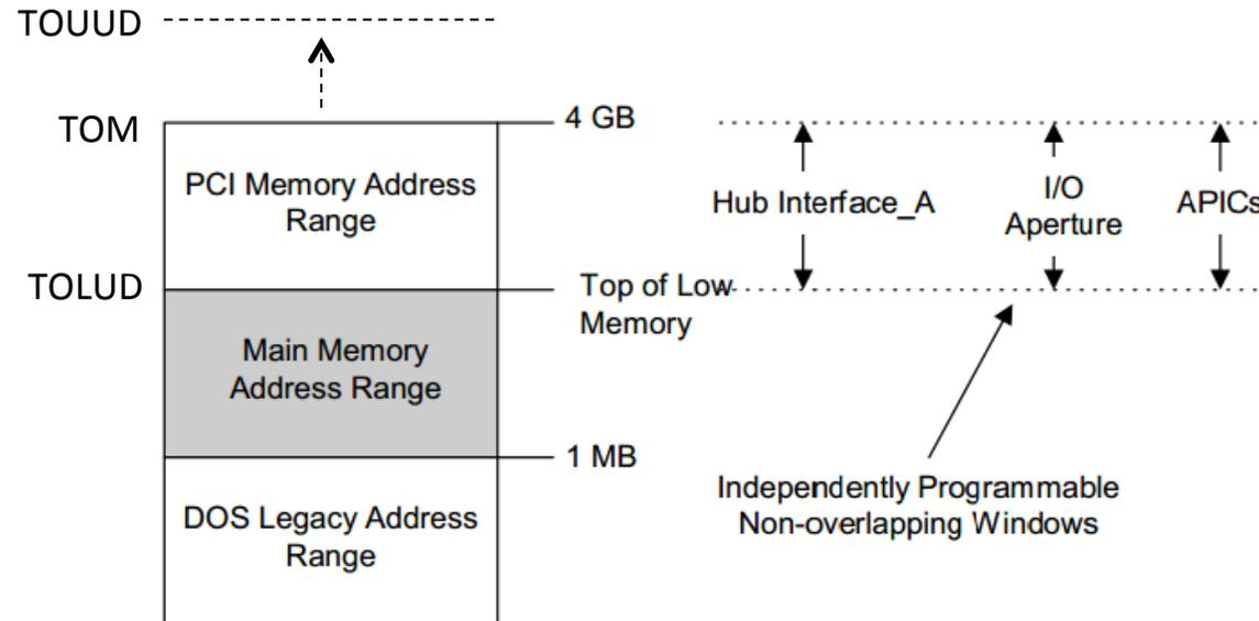
1. High Memory Range: Memory above 4GB (called Top of Upper Usable DRAM). Used for memory mapping and recoverable memory (system memory that overlaps with the PCI range)
